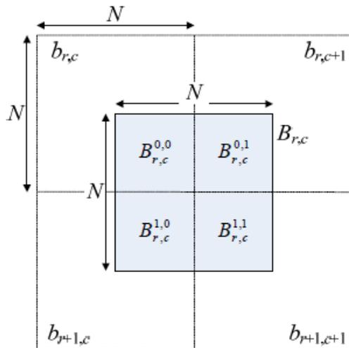
**Figure 2: A De blocking Block (DB) and its Sub Blocks.**
