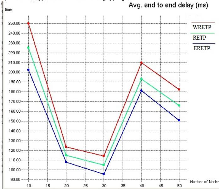
**Figure 6: Shows Comparative result analysis of Average end to end delay graph using without RETP, RETP and Enhanced RETP.**
