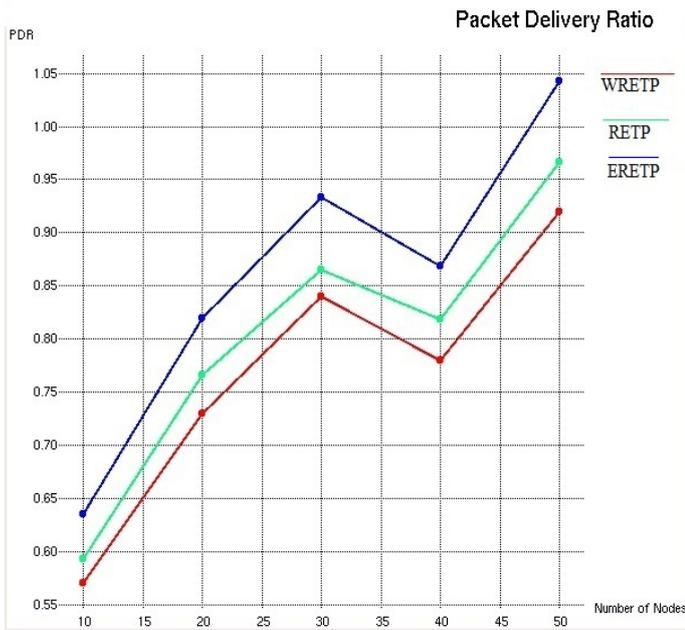
**Figure 5: Shows Comparative result analysis of Packet Delivery ratio graph using without RETP, RETP and Enhanced RETP.**
