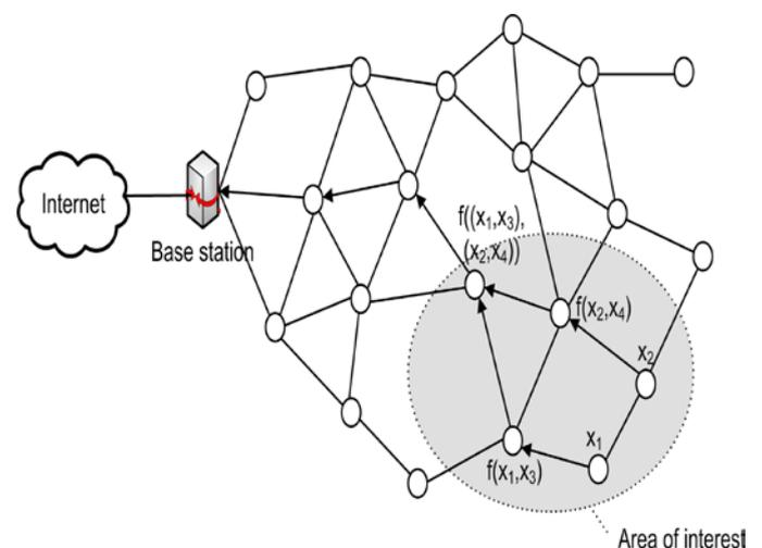
**Figure 1: Wireless sensor network with in-network processing.**
