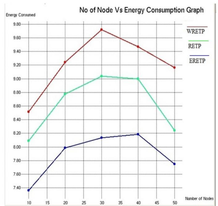
Figure 4: Shows Comparative result analysis of Energy Consumption graph using Without RETP, RETP and Enhanced RETP.
