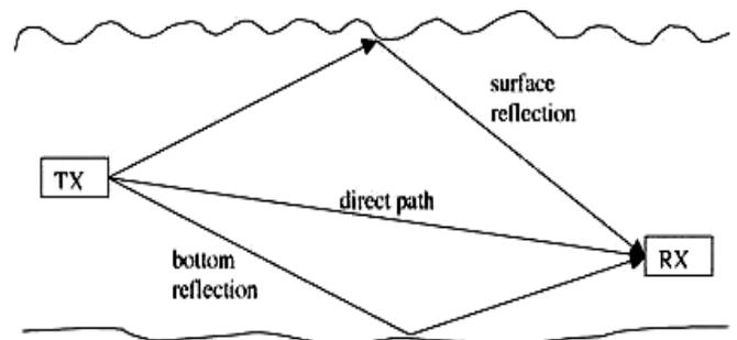
**Figure 1: Shallow water multipath propagation: in addition to the direct path, the signal propagates via reflections from the surface and bottom.**
