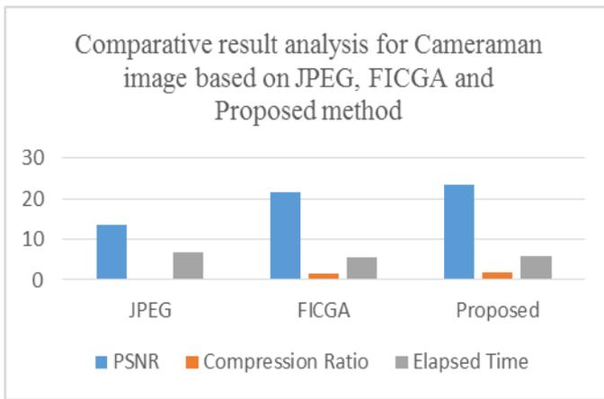
**Figure 7:** Shows that compressed image of camera man based on Proposed method the PSNR value of the image is 23.5604, compression ratio is 1.8834 and elapsed time is 5.7017.
