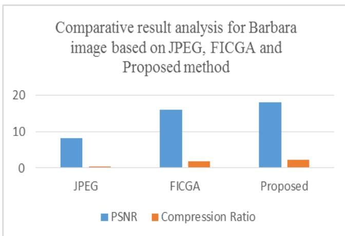
**Figure 9:** Shows that compressed image of Barbara based on Proposed method the compression ratio is 2.1586 and PSNR value is 18.1333.
