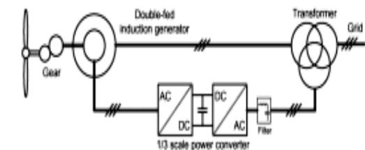
Figure 2: DFIG with partial-scale power converters
