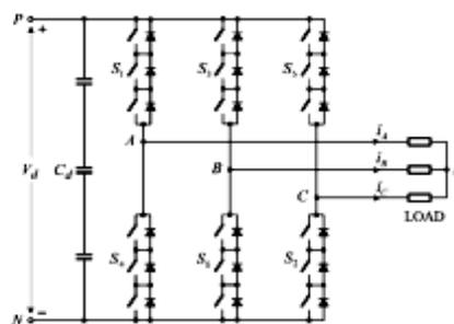
Figure 6: Two-level VSC with series-connected power switches
