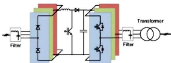
Figure 4: Two-level back-to-back converters with passive rectifier
