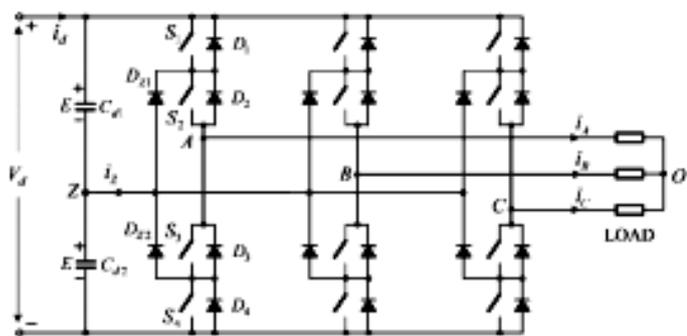
Figure 8: Topology of the NPC converter
