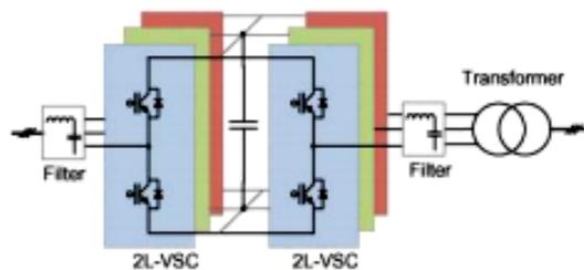
Figure 5: Two-level back-to-back converters with active rectifier
