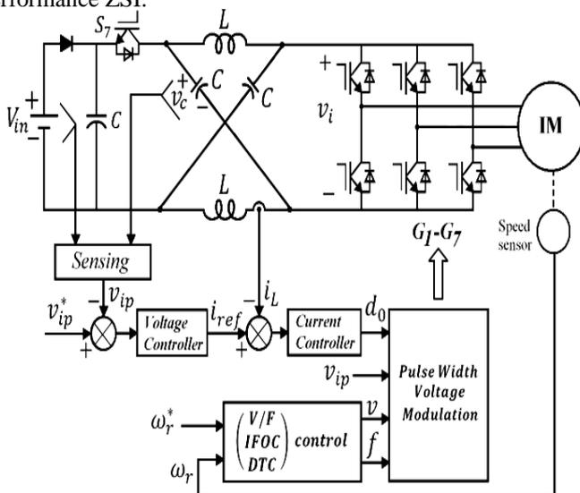
**Figure 4: Closed loop speed control of three phase induction motor fed by a high performance ZSI**
