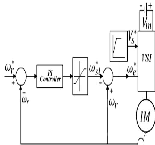
**Figure 1: Block diagram of a scalar controlled induction motor**
