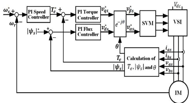
Figure 3: Block diagram of the DTC-SVM based IM drive.
