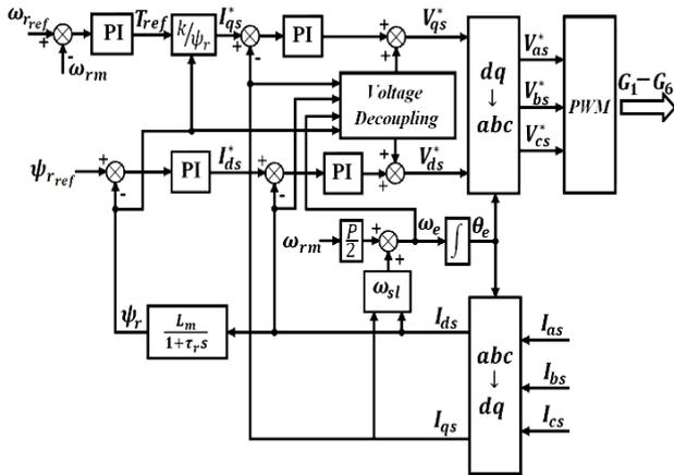
Figure 2: Block diagram of the IFOC of an induction motor
