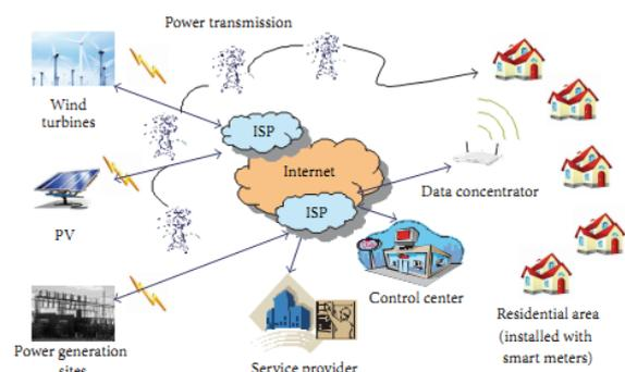
**Figure 1. An example of communication architecture in smart grid.**
