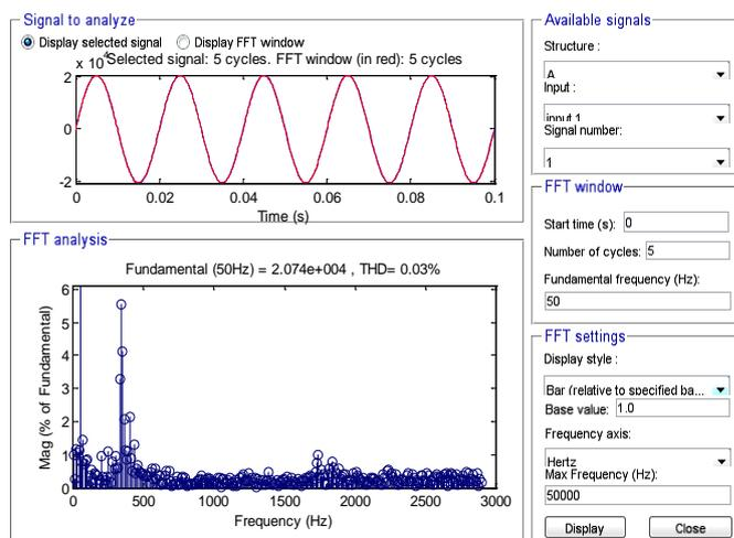
**Figure 9: FFT of Voltage at Load**
