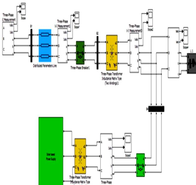
Figure 4: Simulink Model of PV Based grid connected system.
