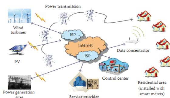
Figure 1: An example of communication architecture in smart grid.
