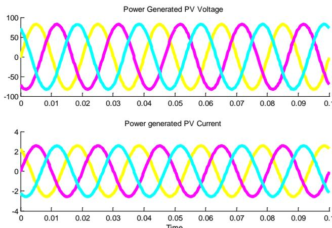
**Figure 8: Voltages and Current Generation of PV System.**
