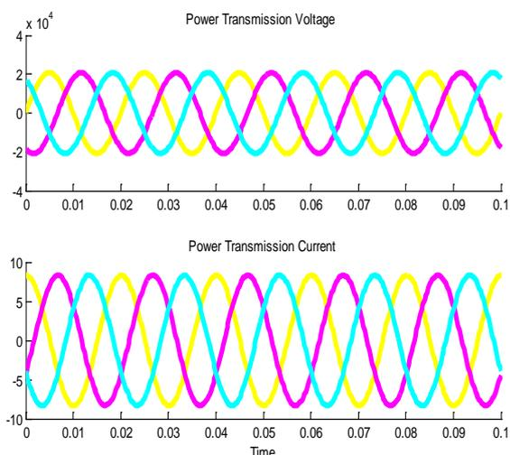
**Figure 6: Grid Voltage and current for transmission.**
