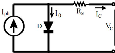
Figure 3: Simplified equivalent circuit of PV Cell
