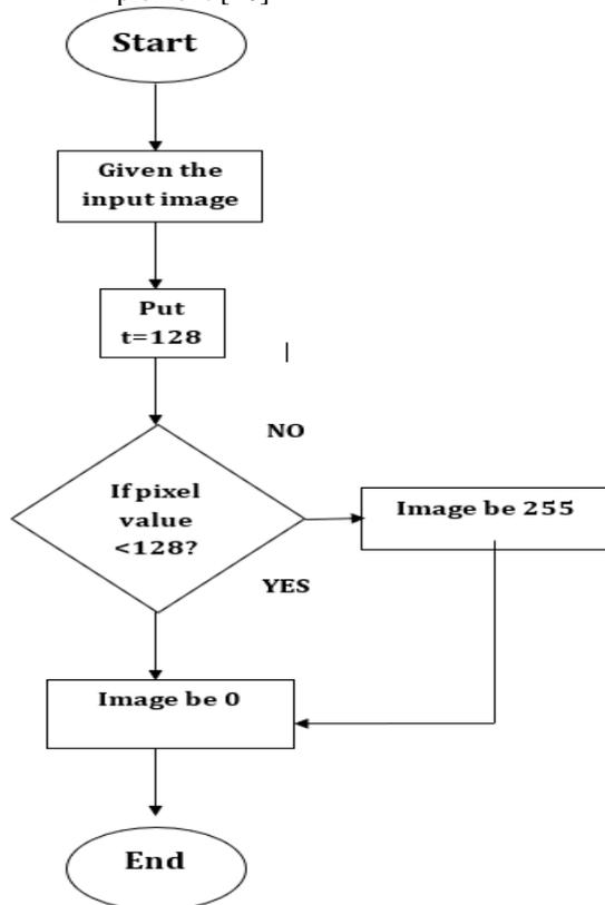
Figure 1: Flowchart of Thresholding Technique.
