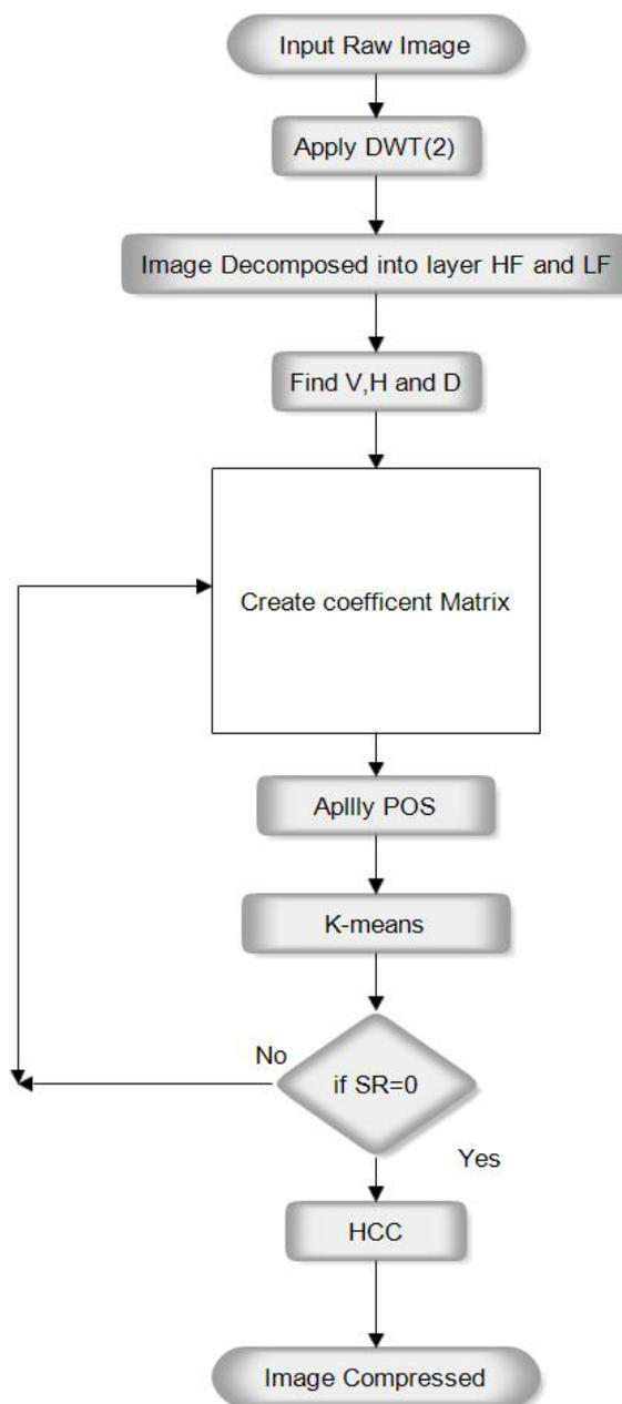
Figure 1: Proposed model of image compression
