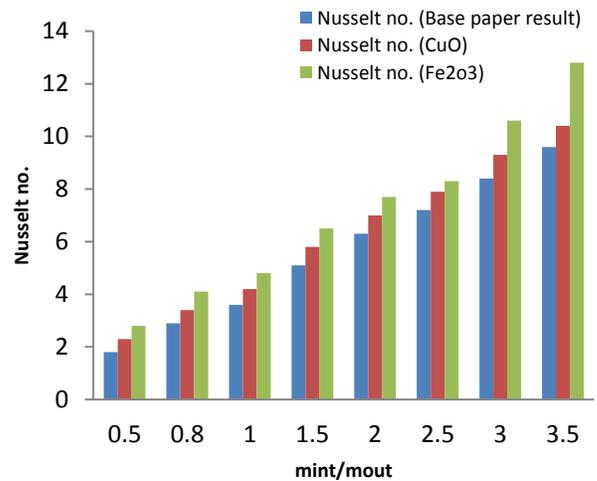
**Figure 7:** Shows the Variation of nusselt no. w.r.t mass flow rate inlet and mass flow rate outlet of different nano fluids and water.
