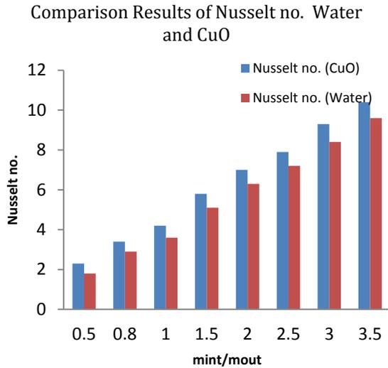
**Figure 4:** Simulation Result of variation in nusselt no. for the helical coil tube heat exchanger with variation in mass flow rate inlet and mass flow rate outlet.
