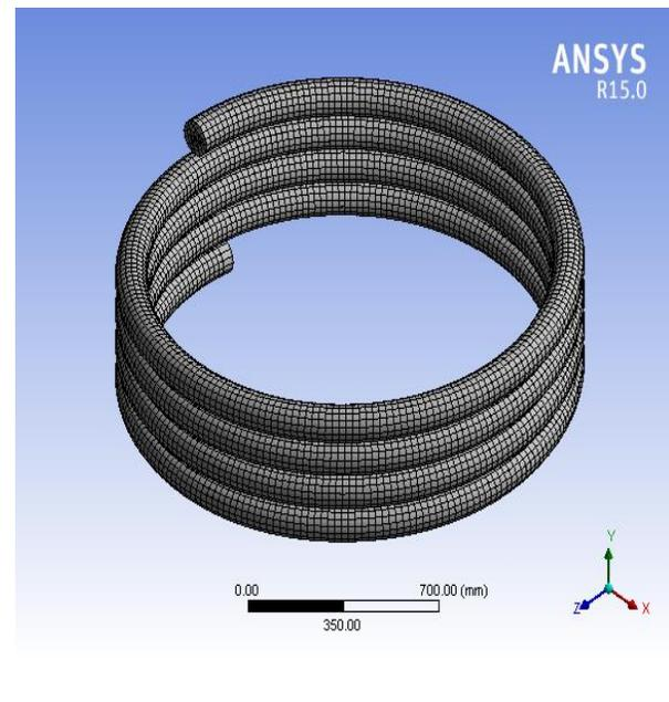
Figure 2: Meshing of Helical coil heat exchanger tube
