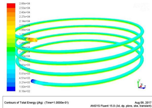
**Figure 5:** Total energy variations on helical coil heat exchanger tube on CuO nanofluid. OVERALL COMPARISON OF HEAT TRANSFER COEFFICIENT AND NUSSULT NO.
