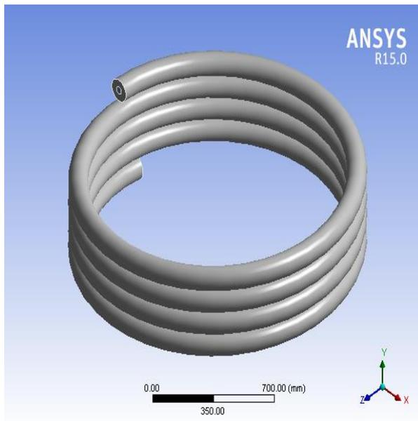
Figure 1: 3D Model of Helical Coil heat exchanger.
