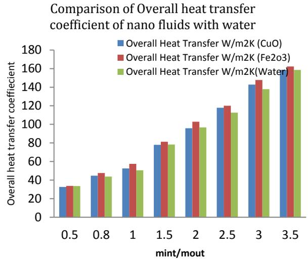
**Figure 6:** Shows the Variation of overall transfer coefficient. w.r.t mass flow rate inlet and mass flow rate outlet of different nano fluids and water.
