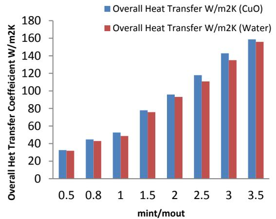
**Figure 3:** shows the overall heat transfer coefficient comparison with water and CuO.
