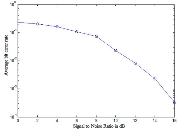
Figure 5: Bit error rate performance of Successive Modulus Matrix.
