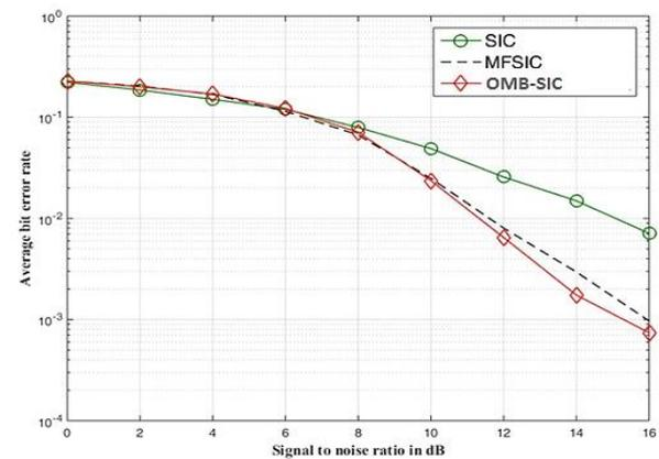
Figure 6: Bit error performance of SIC, MF-SIC and OMB-SIC.
