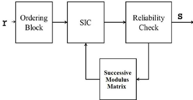
Figure 4: Channel norm ordered Successive Modulus Matrix algorithm block diagram.
