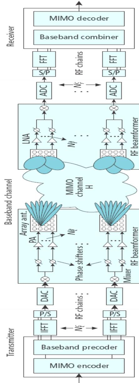
Figure 2: Block diagram of a beamforming architecture.
