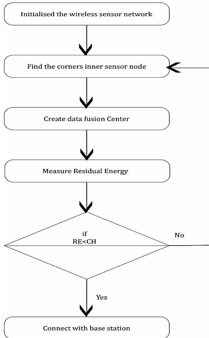
Figure 1: process block diagram of data fusion in cluster based wireless sensor network.
