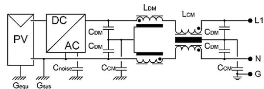
Figure 3: Transformer-less high-input-voltage PV inverter with single-phase common-mode.
