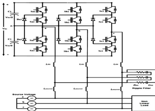
Figure 2: Two and three-level VSI Block.
