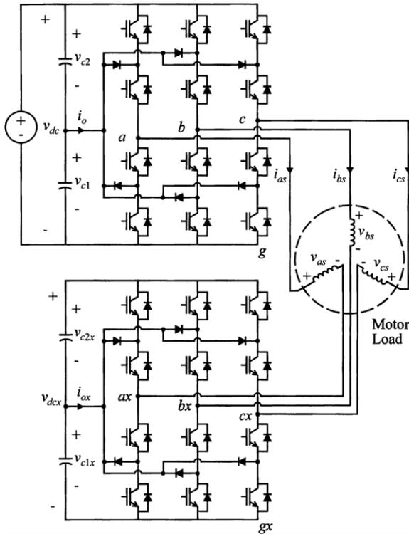
Figure 4: Cascade-3/3 multilevel inverter.
