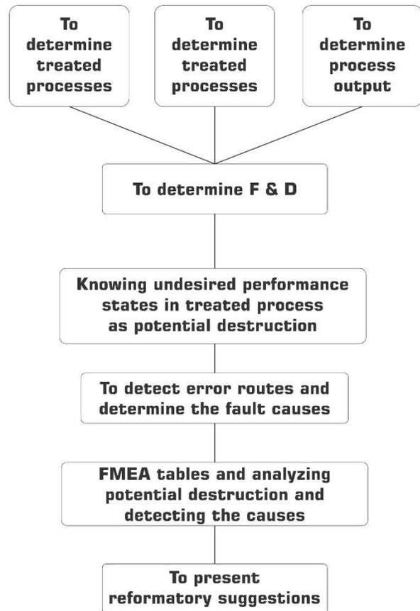
**Figure 1: A Diagram of fault analysis**
