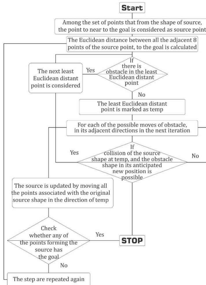
Figure 1: shows that path selection process of fault analysis.
