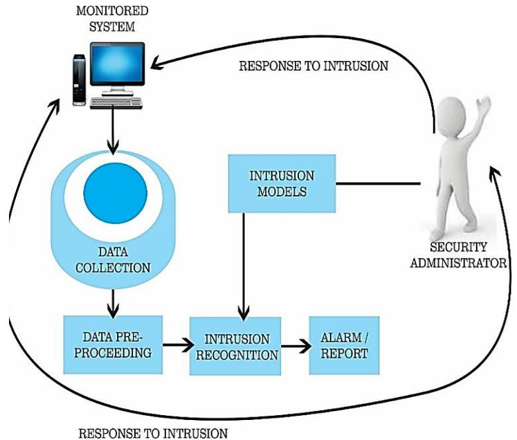
Figure 1: Organization of a generalized intrusion detection system[4].
