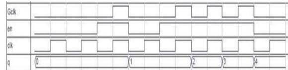
Figure 6: Output of Counter when Counter is Negative edge triggered.
