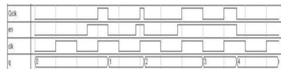
Figure 9: Hazards Problem when AND clock gating Circuitry used.
