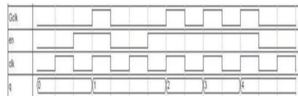
Figure 7: Wrong Output due to Glitch, when counters Positive edge triggered.
