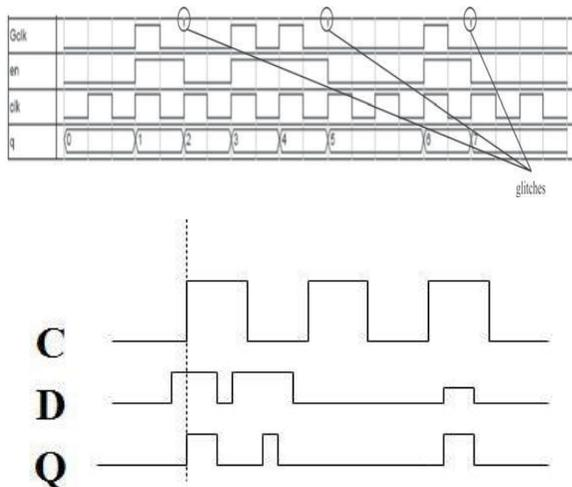
Figure 10: shows that clock time diagram for clock gating
