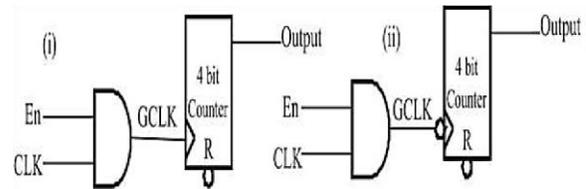
Figure 5: Clock gating using AND gate Circuit.
