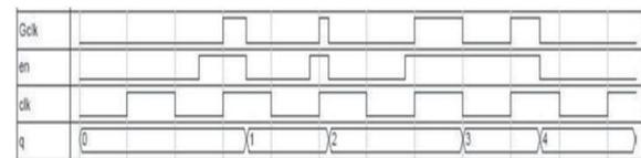
Figure 8: Right Output when counters positive edge triggered.
