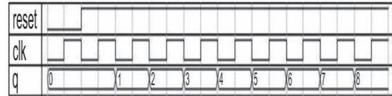
Figure 4: Normal output of the counter without Clock Gating.
