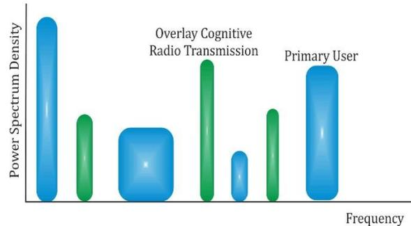
Figure 1: overlay spectrum access mechanism.
