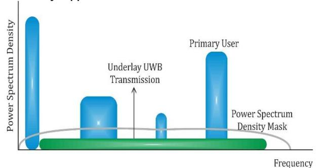
Figure 2: underlay spectrum access mechanism.
