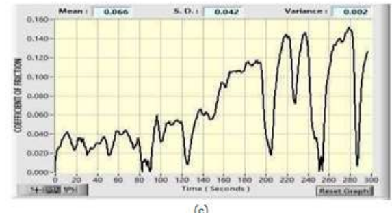
Figure 7: (a) wear, (b) frictional force and (c) Coefficient friction
