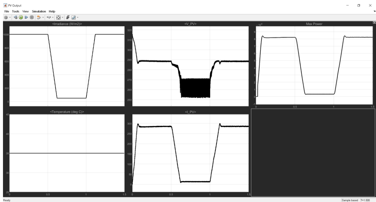
Fig 3. irradiance, voltage, current, temperature, power by Pv vs time
