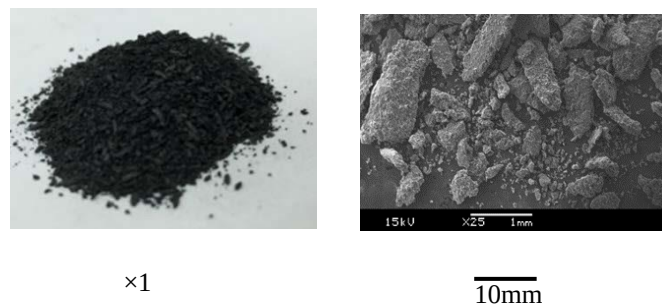
Figure 2. Supplied graphite cutting chips (left) and their scanning electron micrograph (right)
