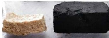
Figure 7. Test pieces sintered in oxidation state (left) and non-oxidation state (right)
