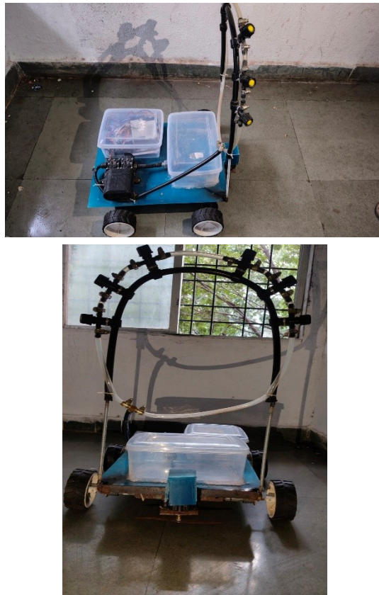
Figure 2 Automated Pesticide Sprayer Machine with Grass Cutter Developed
