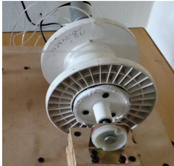
Figure 5 Recycled PET filament collected on a spool.
