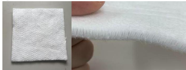
Figure 2. Silica-fiber mat (Belcotex ® ) used in the composite heat insulation.
