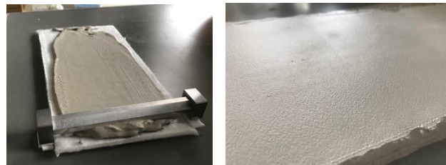
Figure 4. Application of aerogel slurry to the silica-fiber mat using a squeezer technique.
