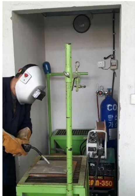
Figure 3. MAG Welding Machine Used for the Experiment
