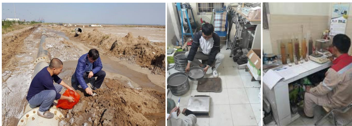
Figure 3. Taking dredged material samples on site and material analysis in the laboratory
