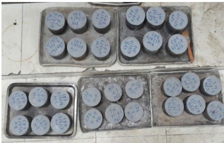
Figure 5. Five group samples of dredged material mixture for foundation of cargo yard
