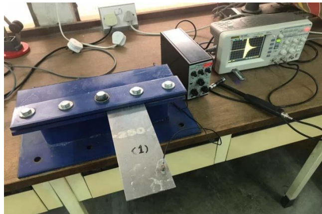
Figure 1. Vibration Rig Compound
